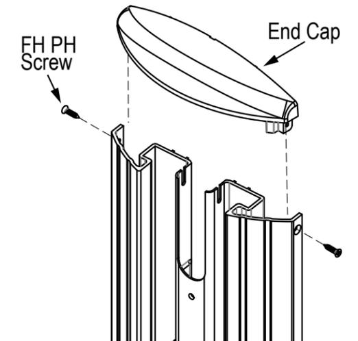
Figure 4.1 End Cap and Actuation Bar Removal
