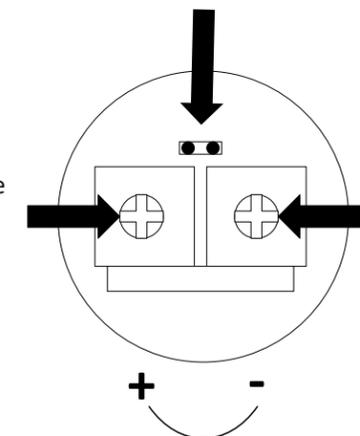
Adjustment for time delay (0.5 to 20 seconds) For Toggle.
