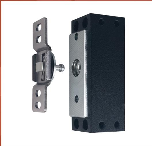
Camden CX-EPD0009 Magnetic Cabinet Lock has an ultra-compact design and is an easily installed high-security lock for virtually any enclosure door, including computer cabinets, refrigerators, lockers, and retail display counters. This 12V or 24V magnetically operated lock has a holding force of 440 lbs. (200 kg) and is water-resistant, making it ideal for humid environments, including inside fridges and freezers.
