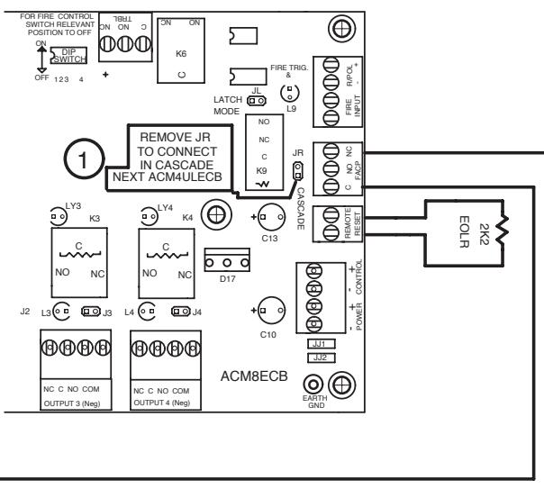
Maintain a minimum distance of 0.25 inches between power-limited and non-power-limited wiring to prevent electrical interference.
