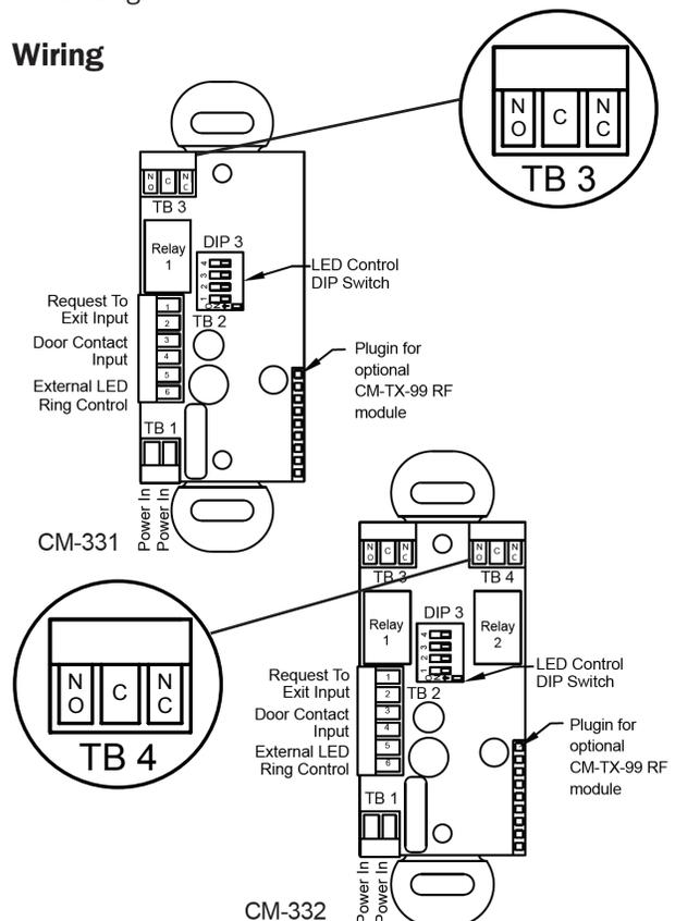
**Caution:** Do not apply power to the unit until all secondary wiring is complete, and dip switches have been set.
