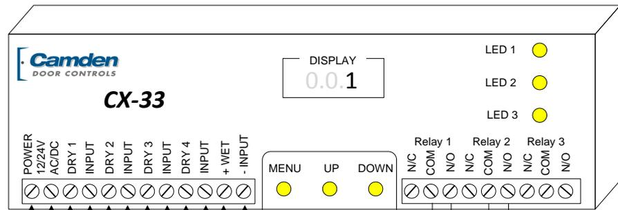
NOTE: Each of the 4 dry inputs can produce a different output result. This drawing shows all possible Input types, (any or all may be used). This is called Mixed Mode Triggering.
