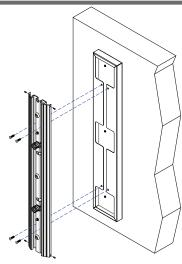
**Note:** When reinstalling the actuation bar, make sure the hanger fits snugly into the slot.
