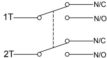
**Momentary:** When the switch is pressed it will provide a change of state on both of the N.O. & N.C. poles until released
