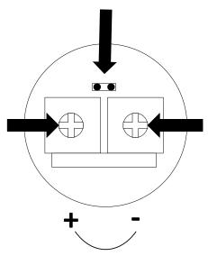
Adjustment for time delay (0.5 to 20 seconds) For Toggle. Turn clockwise to increase time delay
